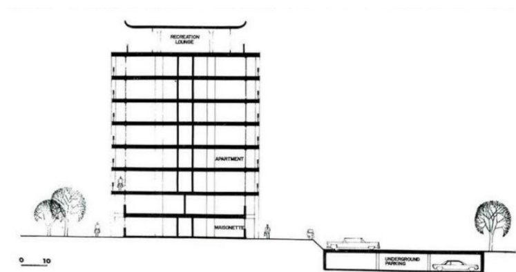
Figure 39: East-west section through 1 Deauville Lane showing general construction details (Source: Grossman 1961:62).
