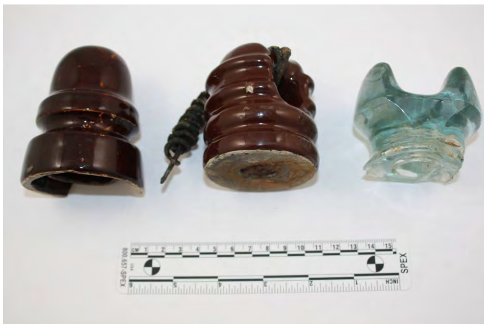
Plate 102: External electric insulators. Left, porcelain pin type insulator from Lot 301 (Cat. #12700); centre, porcelain wire holder insulator from Lot 385 (Cat. #11980); right, glass saddle insulator from Lot 301 (Cat. #9995).
