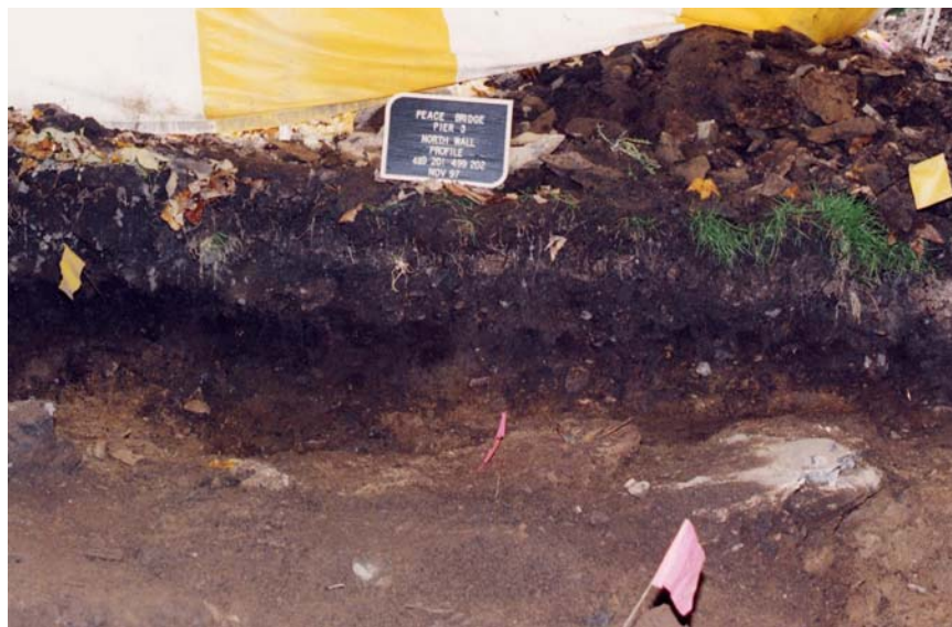
Plate 4.6: The paleosol, sand subsoil and bedrock in Pier 3.
