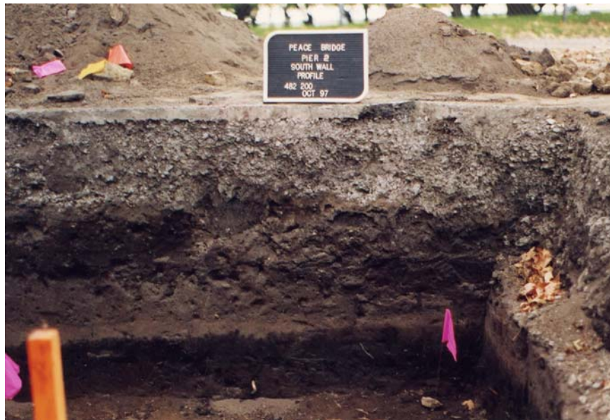
Plate 4.1: The general stratigraphy encountered in Pier 2—asphalt and granular over disturbed topsoils over upper paleosol over sand horizon over lower paleosol formed on subsoil.
