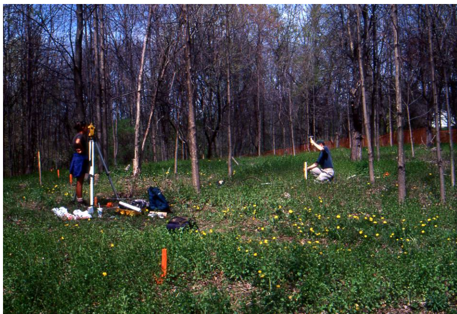
Plate 1: Setting up the recording grid using the 500N-200E datum stake.
