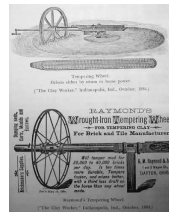
A circa 1884 advertisement for a tempering wheel used in a ring pit (Weiss and Weiss 1966)
