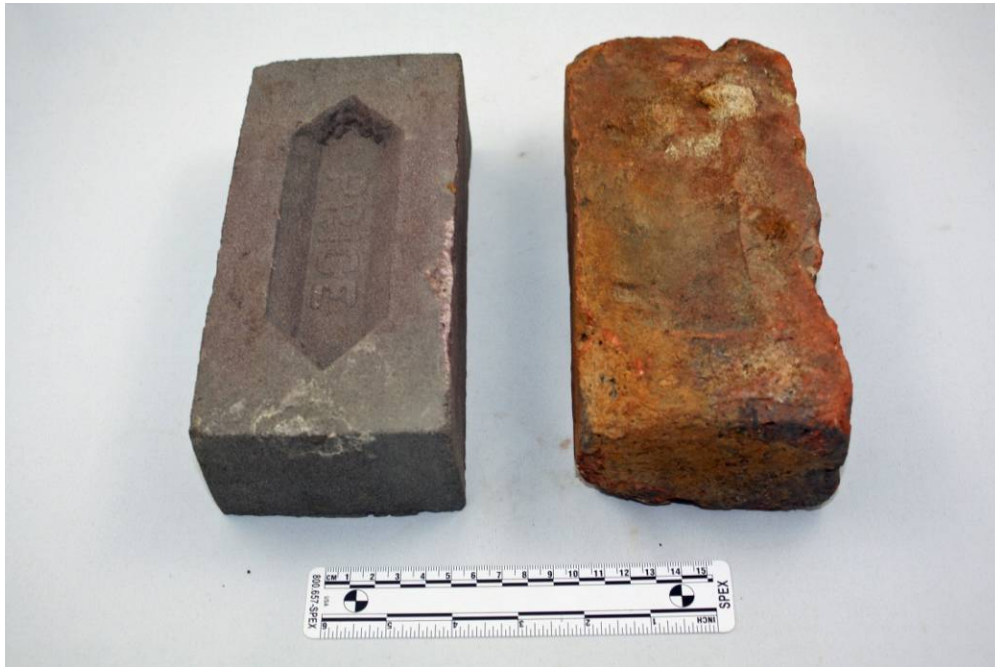
Plate 77: Left, PRICE brick with a hexagonal frog from Lot 59 (Cat. #805). Right, hand-made brick with a shallow rectangular from Lot 5 (Cat. #670).
